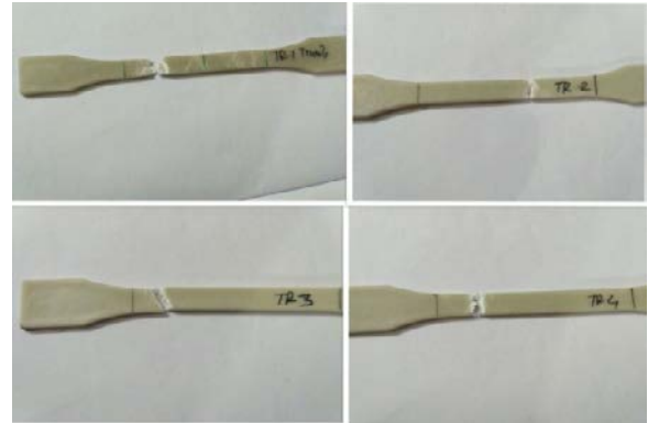
Fig 2: Tensile specimen after testing
